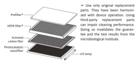
\* HEPA filters and prefilters are a part of this device model.
